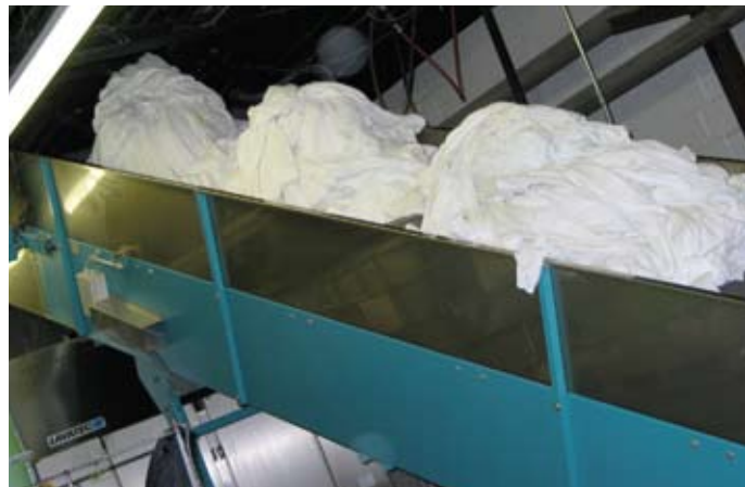
Employees in the finishing department feed textiles into a flatwork ironer; finished, folded goods are prepared for packout; two of several large dryers; two water softening units; soiled goods head up a conveyor and into the tunnel washer.
